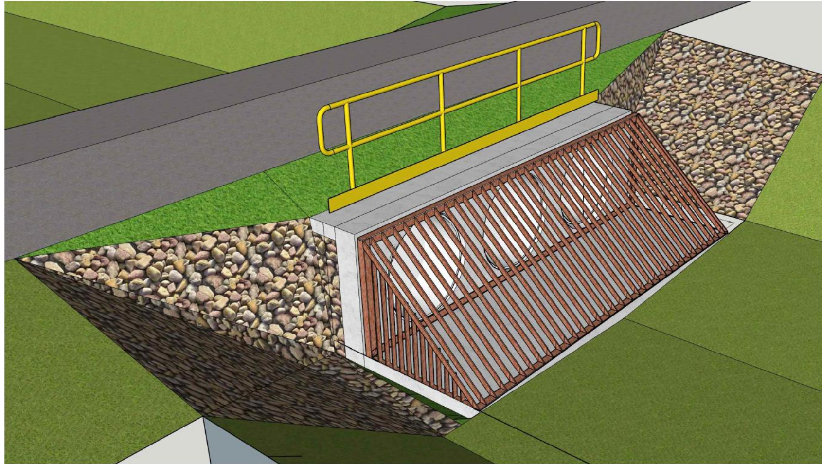
CULVERT CROSSING CS-04 DETAIL A - PERSPECTIVE VIEW SCALE: N.T.S.
