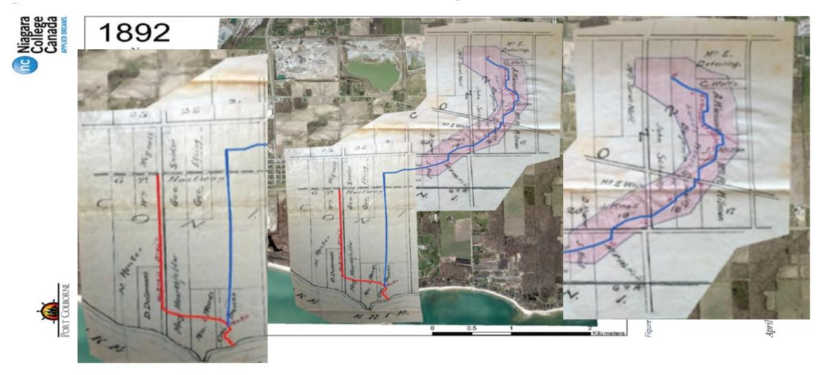
By 1927 the west branch of Wignell (W1) and Michener M2 were extended to Second Concession Road, and the Michener M2 drain was connected to the Wignell main drain to utilize the larger capacity crossing under the Canadian National RR (CN) tracks
