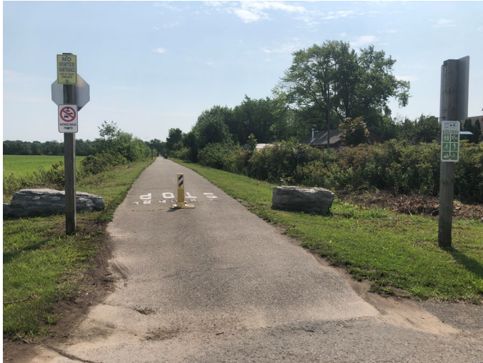
Bollard Crossings, the standard crossing that appears at low-traffic rural crossings
